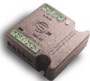
Bus Enabled, 2channel Relay module 5 Amp per channel for Automation Security Siren, Electric Lock, Curtain motor, trigger of gate/Garage Motor, Lighting control, ... etc. (Built in Intelligence and delay and double throw Function) - Small size can fit behind switch. With Broadcast Enabled, Ready with Firmware USB Upgrade
